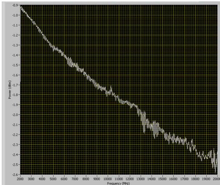
Figure 1: Cable losses without any correction applied
