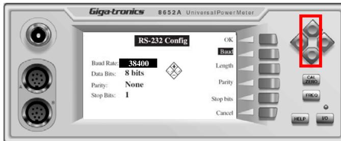
Figure 7: Configure the RS-232 settings
