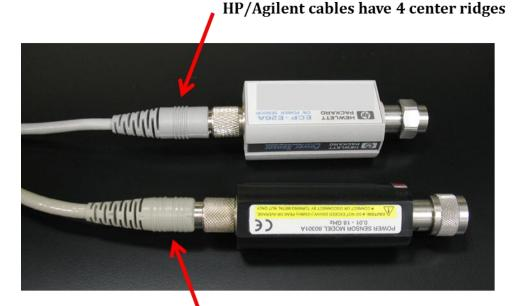
Giga-tronics cables have 6 spread-out ridges
